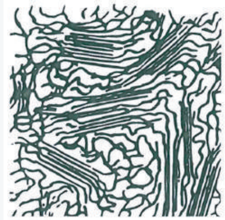
Molecular structure of semi-crystalline plastics: solid molecules have a partially crystalline structure
